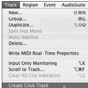
Figure 3-10: Choosing Track ⇨ Create Click Track creates a track with the click inserted.
