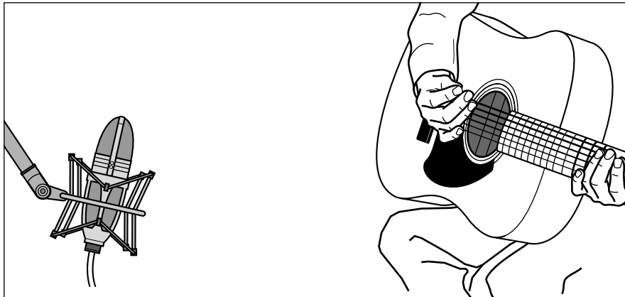
Figure 2-2: Distant miking places a microphone three or four feet from the sound source.
