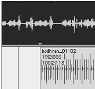
Figure 3-8: You can align the synch point from one region to the start point of another.
