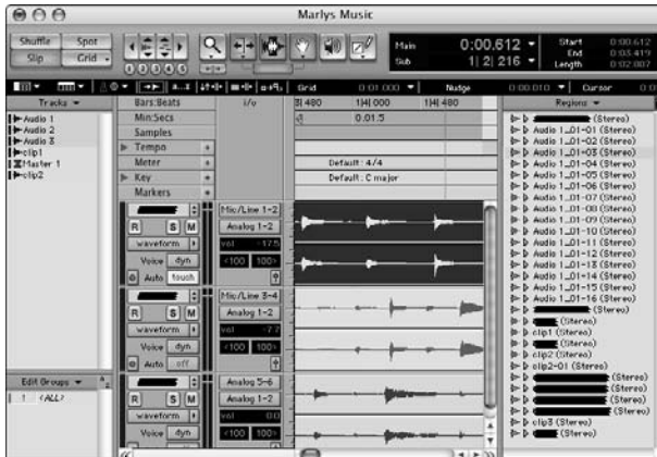
Figure 1-6: To show the Show/Hide Tracks list, click the arrows in the lower left of the Edit or Mix windows.
