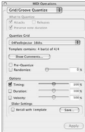
Figure 4-5: The Grid/Groove Quantize function lets you align your notes to a groove template.
