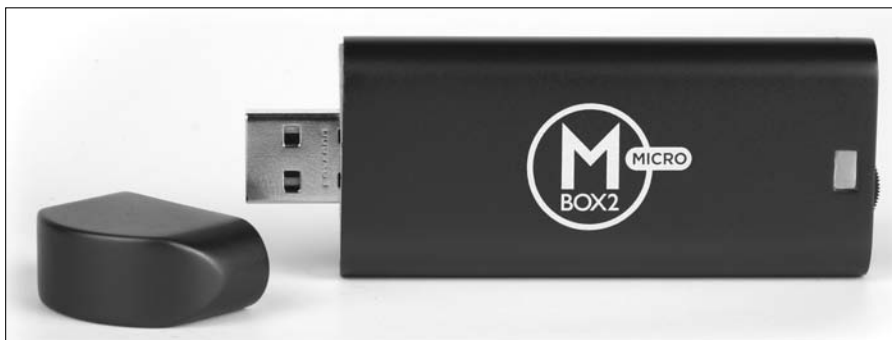
Figure 2-1: The Mbox 2 Micro is a tiny output-only device for working on your tracks.
