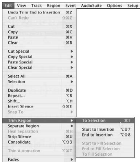
Figure 3-2: Use the Trim to Selection command to get rid of unselected parts of a region.
