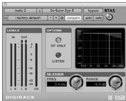
Figure 4-5: Use the De-Esser plug-in to get rid of unwanted sibilance.
