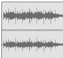
Figure 3-21: A stereo track (top) can be split into two mono tracks (bottom).
