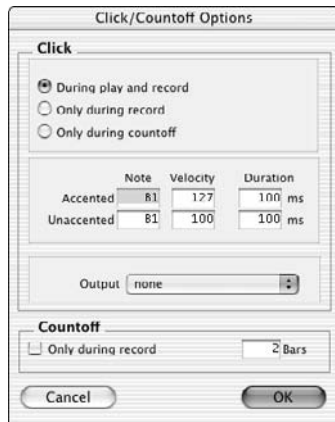
Figure 3-11: Use the Click/Countoff Options dialog box to configure your click track device.
