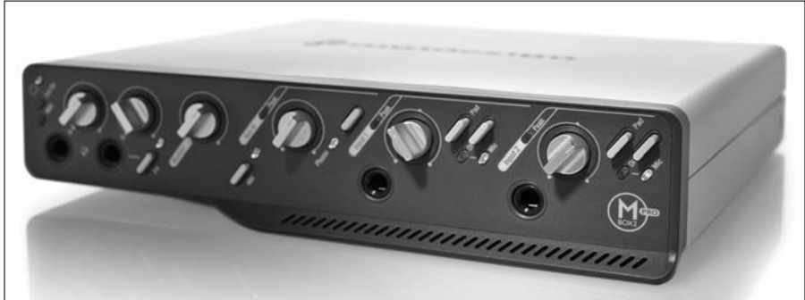
Figure 2-4: The Mbox 2 Pro is a portable FireWire interface with MIDI capabilities and a bunch of Pro features.
